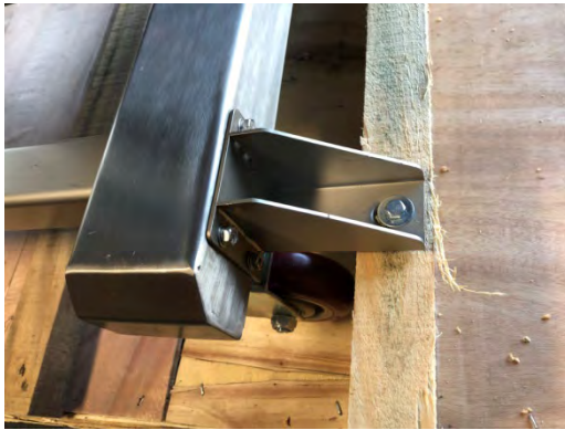
Figure 6. Bolts locking HL-M1120LD to crate.
