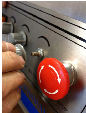
Figure 27. Remove Ink Temperature Knob
